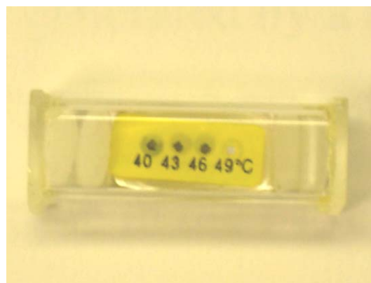
Fig. 1. Temperature measurement is based on temperature indicator strips. The strip is attached to the surface of the glass slides and sealed in the glass tube. The accuracy of the indicator is \pm 1 °C. Here, the strip indicated that the maximum temperature of the sample reached between 46 and 49 °C. This is reported in Table 1 as 47.5 \pm 2.5 °C.
